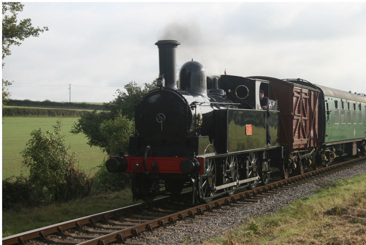
Below: LNWR 0-6-2T Coal tank. 300 were built between 1881 and 1887. They were a tank version of the LNWR Webb Coal Engine. 1054 was the 250th built in 1888.
