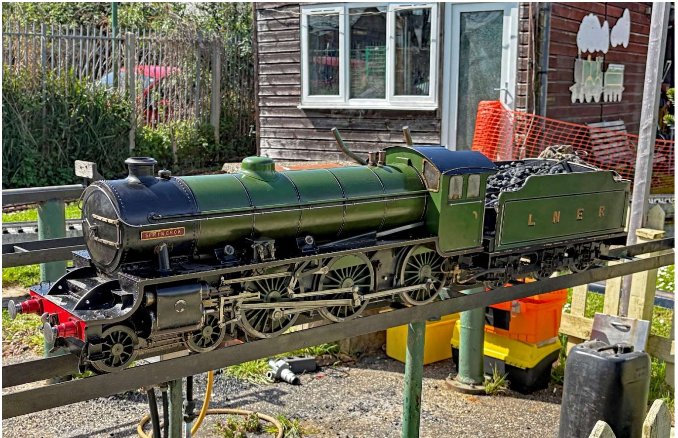
BR 4-6-0 class B1 SPRINGBOK steam loco on the raised working area to allow the fire to be raked and take on water and coal.
