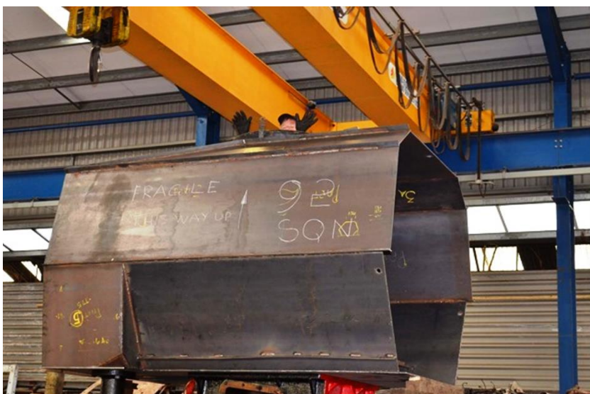
This is the replacement smokebox, built using my cleaned-up scrapped box as a pattern.
