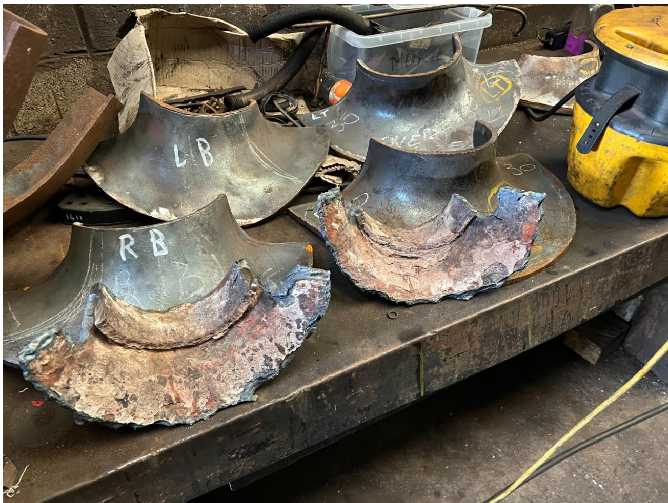
Removed sections of collar, showing wasting and heavy scale with replacements suitably labelled.
