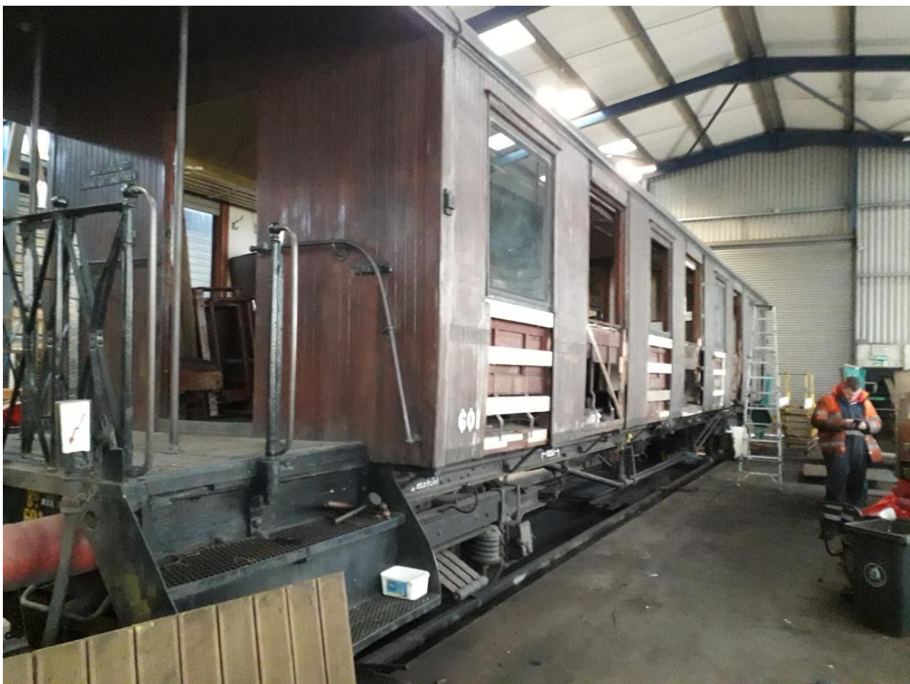
The Norwegian coach, showing some of the new softwood supporting timber, replacing rotten original timbers.
