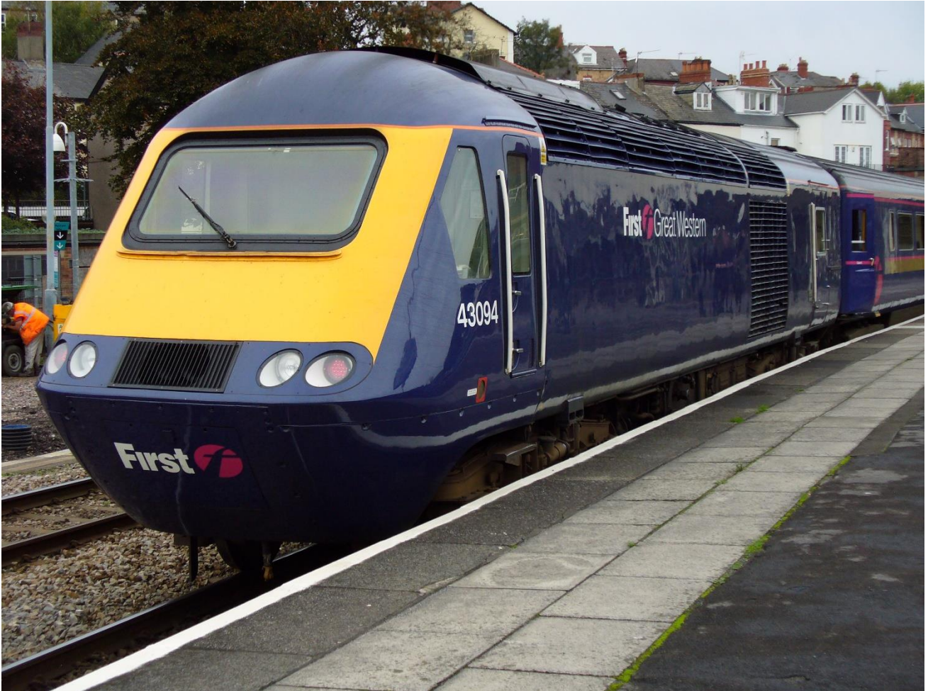
First Great Western's 43094 - at Casnewydd (otherwise known as Newport), South Wales on 23rd October 2006. The power car had been recently outshopped in the, then, latest FGW livery and had also just been fitted with an MTU 16V4000 power unit.
