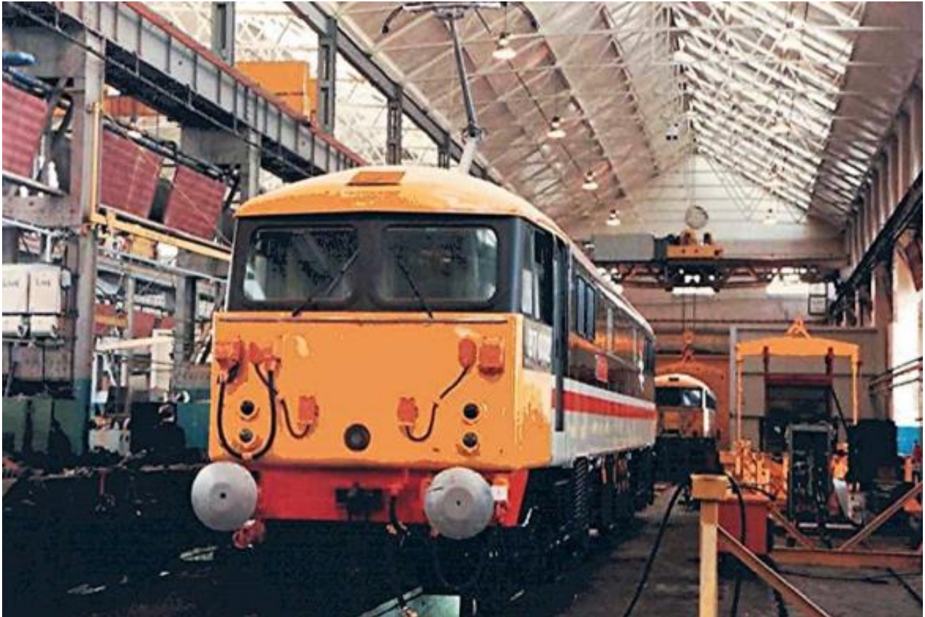
Class 87 in the TRS/Major Depot north bay, looking west (pan up!). This was probably nearing the end of a CEM overhaul. 40-ton crane in the background.
