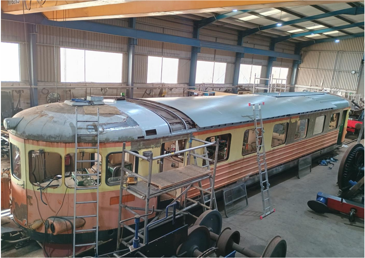
Replacement roof taking shape (12 February)
