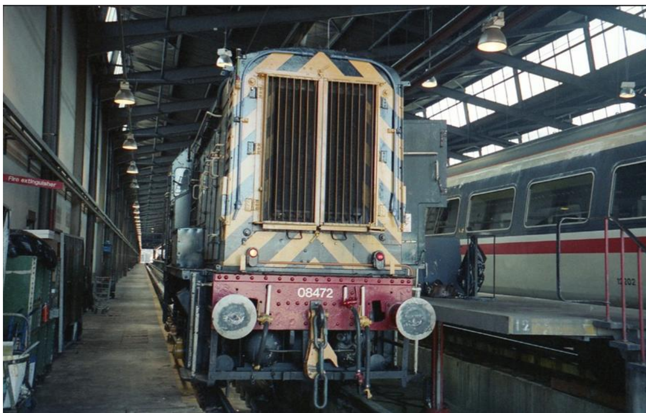
08 472 on 12 Road, receiving attention. Note the raised platform and side pit below between 12 road (left) and 11 Road (right), and underside pits. The 08 is also fitted with a tightlock coupling adaptor (behind the 3-link coupler) for use with Mk4 coaches split from within a set. Photo: David Burrell.
