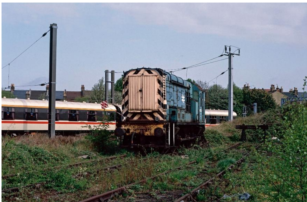
A view of 08 222 on the former Palace Gates sidings at the north end of the depot. This loco was vacuum braked only, so was withdrawn in 1984 and lingered on-depot for around another 12 years. Note the white-roofed Mk1 charter stock behind. Photo: Adrian Nicholls
