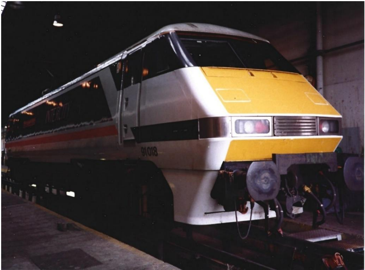
A final view of 91 018 on 13 road, on the author's last day at Bounds Green, May 1994. Note the modified horn grille and sealed covers over the nose end jumper cable connections, just above the head/tail lights. Photo: Hugh Driscoll.
