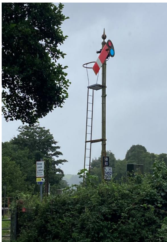
GWR pattern lower quadrant signal SB40, in the OFF position, permitting the Newquay branch train (a class 150) to proceed from Par to Newquay. Note the footpath crossing.
