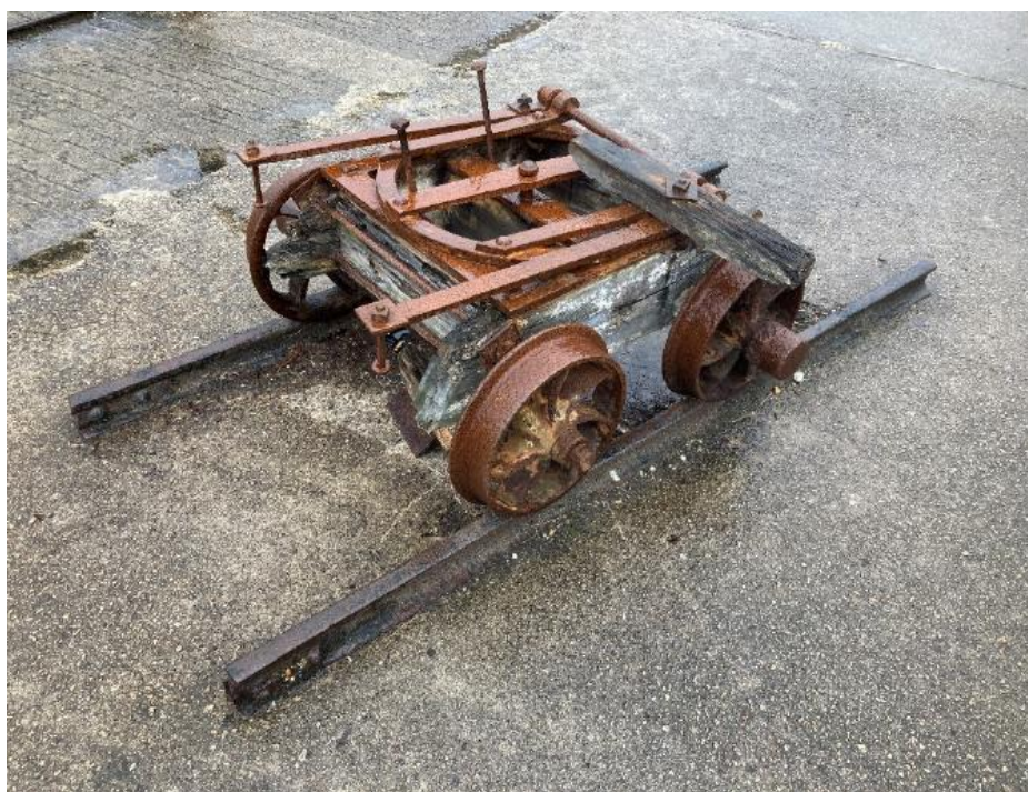
Charlestown Harbour Tramway wagon bogie. It appears that the wagon body would have been capable of rotation and tipping.
